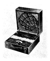
**▼HE McMichael model SMC Suitcase** Portable receiver employs a 4-valve battery-operated chassis having a valve arrangement comprising a tetrode RF amplifier, a triode detector, a triode first AF amplifier and a pentode output valve. The receiver has provision for an external aerial and earth and for headphones.
